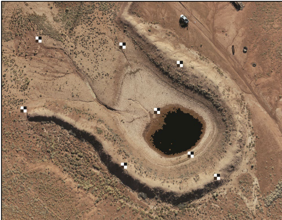
Example of Ground Control Point (“GCP”) Placement at Points of Interest for an Impoundment
