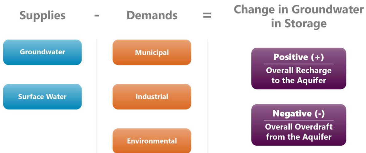
Figure 2. Depiction of the Bonita Creek water budget, including all available supplies and demands and how they contribute to changes in groundwater in storage.
