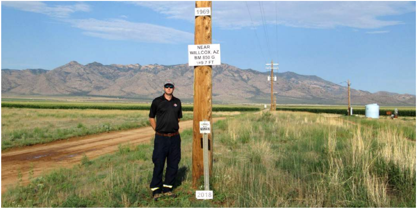
This photo shows the approximate land surface in 1969 and 2018, with nearly ten feet of land subsidence over that time period.
