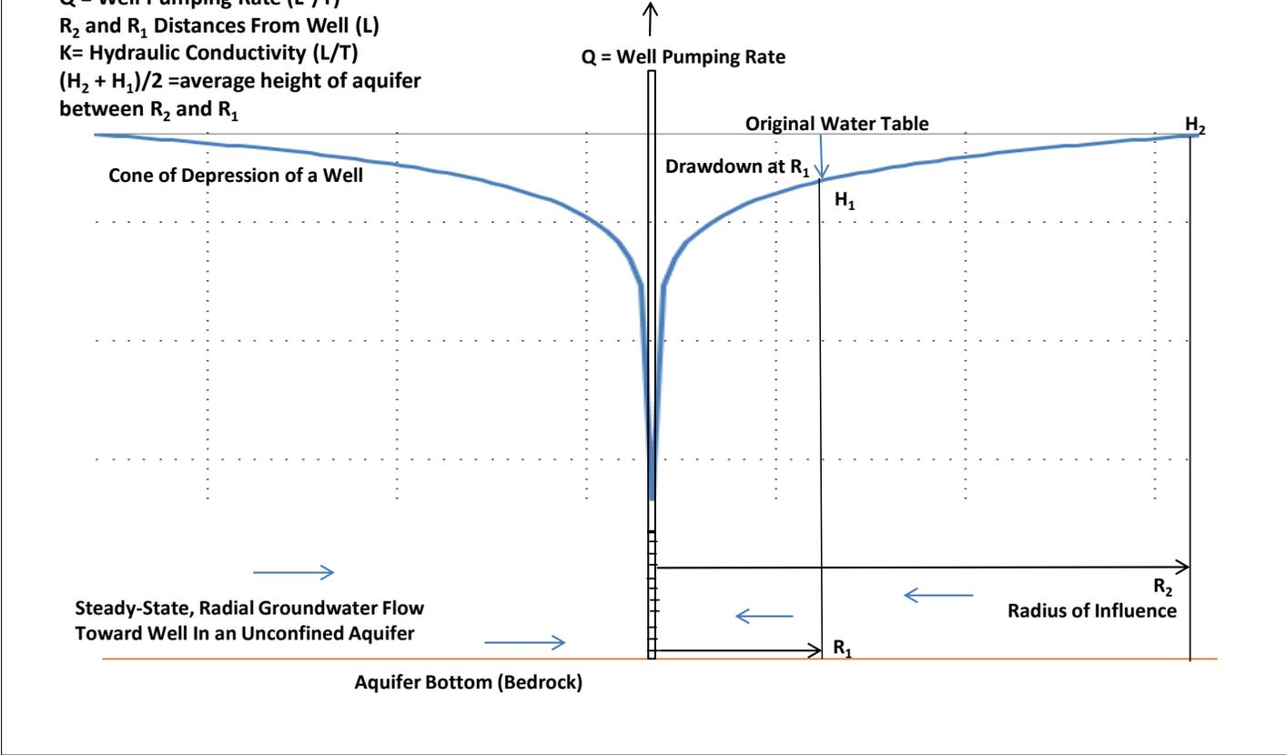
**Figure 2** Thiem Equation For Steady-State Radial Flow In An Unconfined Aquifer
