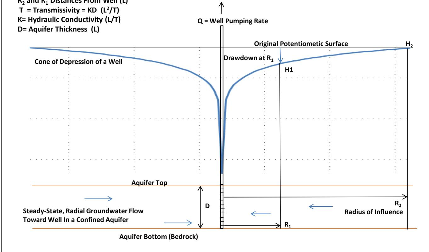
**Figure 1** Thiem Equation For Steady-State Radial Flow In A Confined Aquifer
