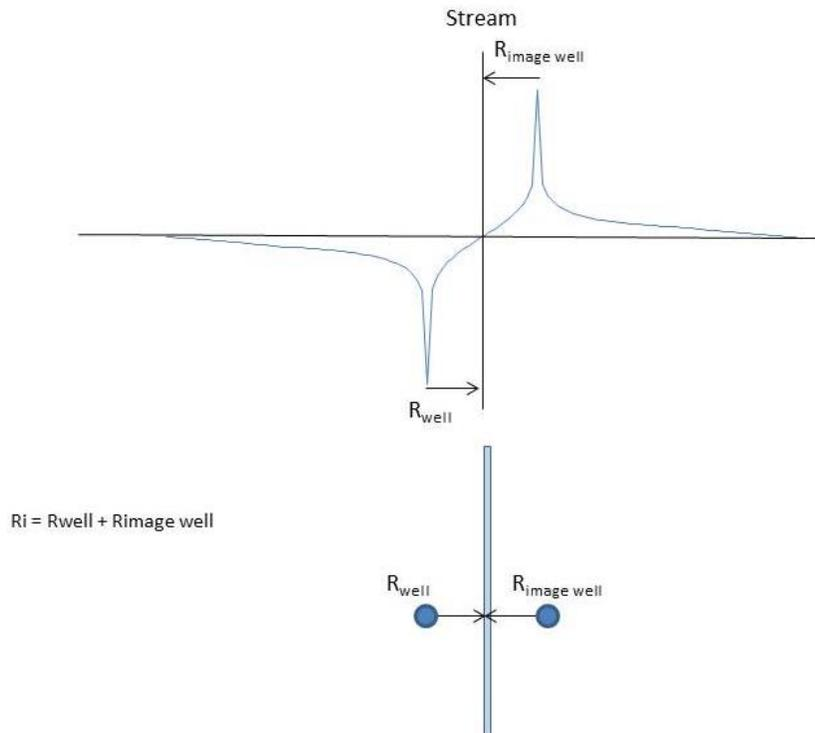
**Figure 4** Application of Superposition to Simulate Drawdown From A Well Near A Stream
