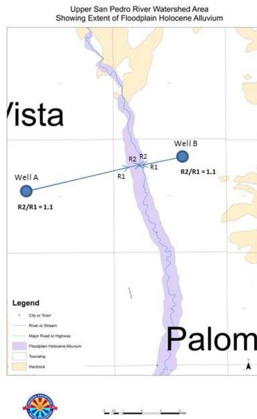
**Figure 7** Map Showing  $R_2/R_1$  Distances Vary Due to Subflow Zone and Stream Geometry
