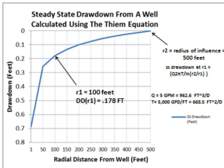
**Figure 5** Theoretical Steady-State Drawdown of a Well Calculated Using the Thiem Equation
