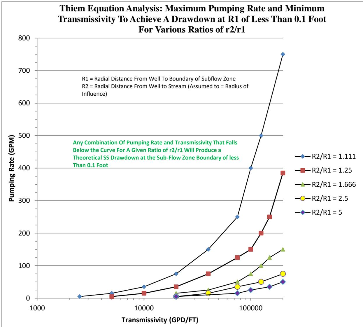
**Figure 6** Maximum Pumping Rate and Minimum Transmissivity to Achieve a Maximum Drawdown of 0.01 feet at R<sub>1</sub> (Sub-flow Boundary) For Various Ratios of R<sub>2</sub>/R<sub>1</sub>
