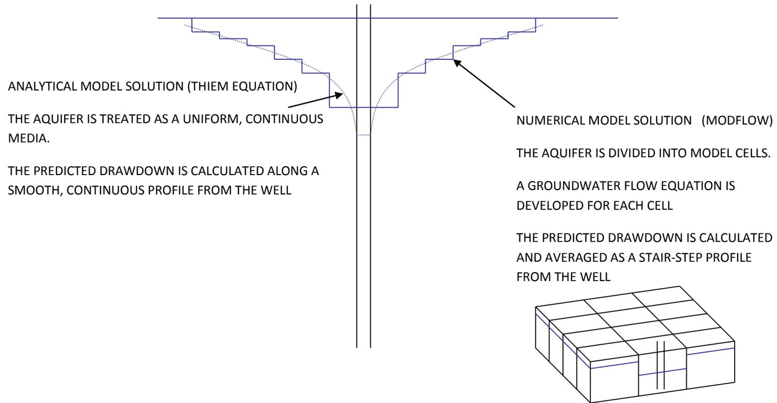
**Figure 12** Comparison of drawdown simulated with analytical and numerical groundwater models
