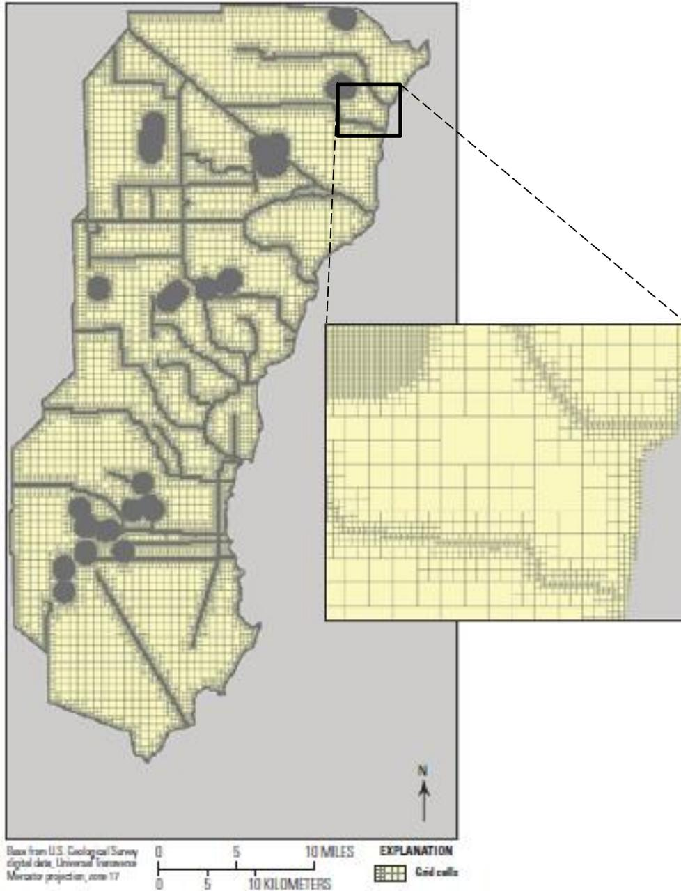
**Figure 13** Example of grid cell variability provided using MODFLOW-USG in a groundwater model of Biscayne Bay (USGS Techniques and Methods 6-A45)
