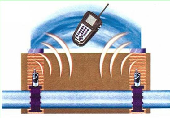
**Leak Detection System.** Magnetized Units transmit leak status signals to Patroller unit
